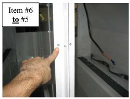
Tighten screws holding **Rear Doorframe** to **Center Divider**
